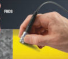
Duplex Probe measures individual layer thicknesses of zinc and paint in a duplex coating system
